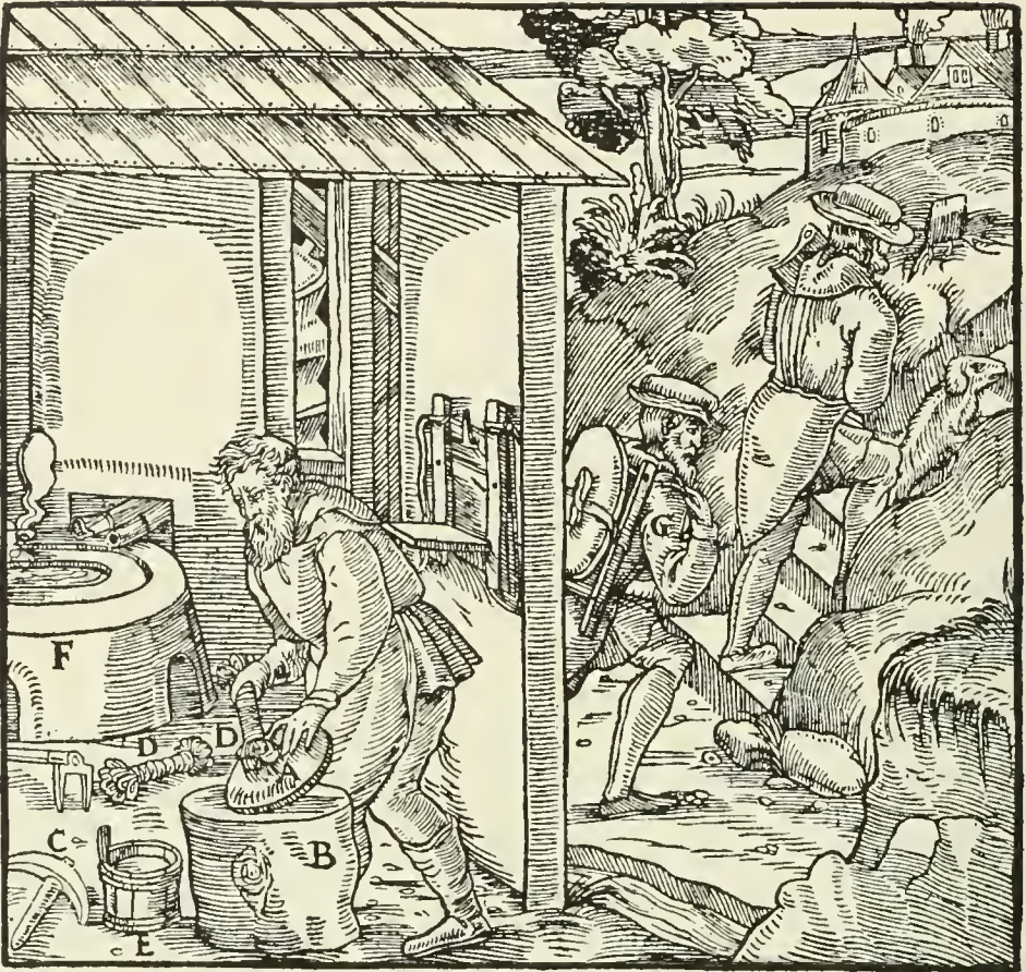
A—CAKE. B—STONE. C—HAMMER. D—BRASS WIRE. E—BUCKET CONTAINING WATER. F—FURNACE FROM WHICH THE CAKE HAS BEEN TAKEN, WHICH IS STILL SMOKING. G—LABOURER CARRYING A CAKE OUT OF THE WORKS.
